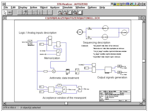
Figure 8: Smart Sensor With Autocalibration And Non-Linear Capabilities
