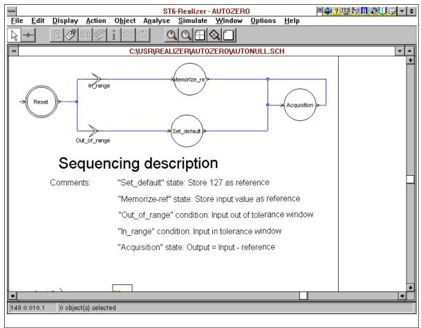
Figure 7: Sequencing Description By State Machine
